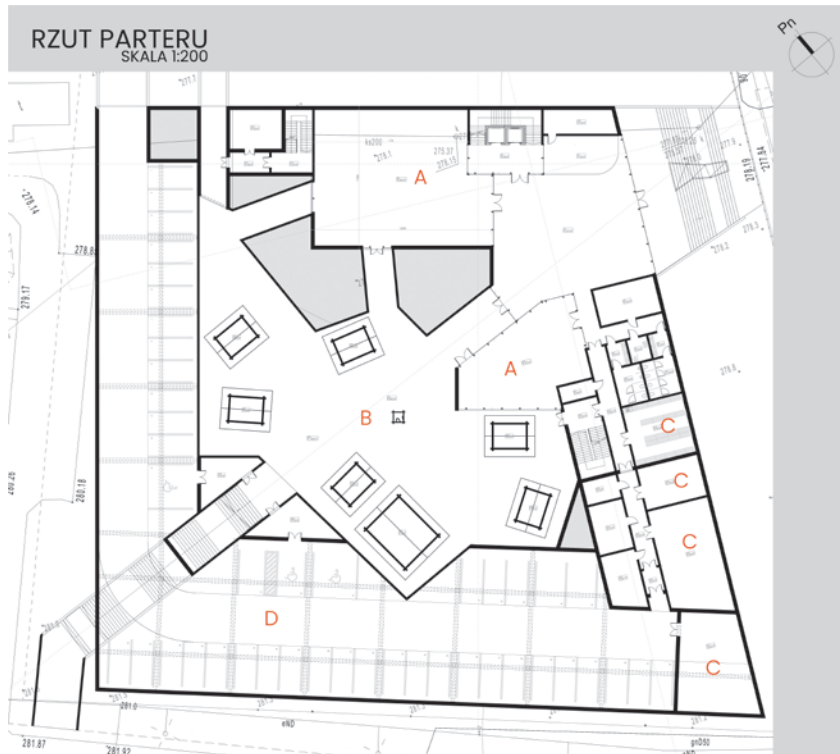
Fig. 2. Project of the Archaeological-Historical Centre “Cherven’ Towns” – ground floor plan (A – exhibition halls; B – courtyard with the reconstruction of the fragment of the ward; C – storehouses; D – parking)
